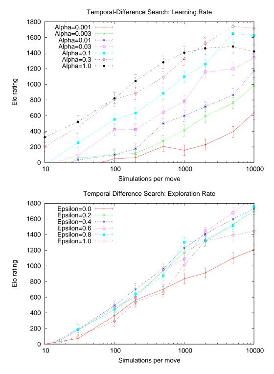
Figure 6.4: Performance of temporal-difference search with different learning rates  $\alpha$  (top) and exploration rates  $\epsilon$  (bottom).
