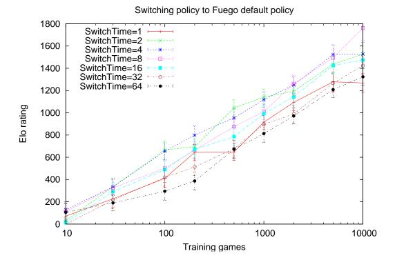
Figure 6.2: Performance of temporal-difference search when switching to the *Fuego* default policy. The number of moves at which the switch occurred was varied between 1 and 64.
