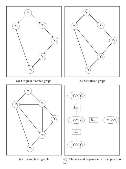
Figure 3.3: The Junction Tree algorithm
