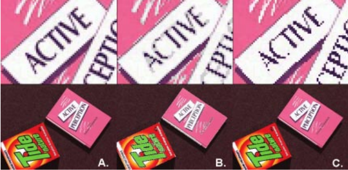
Figure 7: The dominant colors identification algorithm is applied to the sample image shown in A. On the top, portion of the result image is amplified for display. A. The original image. B. The image with only dominant pixels, all other pixels are grey. C. The image with both the dominant pixels and the transitional pixels that assume a dominant color.
