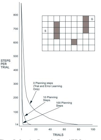
Figure 7. Learning Curves for Dyna-AHC Systems on a Simple Navigation Task. A trial is one trip from the start state "S" to the goal state "G". The more hypothetical experiences ("planning steps") using the world model, the faster an optimal path was found. These data are averages over 100 runs.
