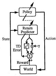
Figure 4. Adaptive-Heuristic-Critic Architecture. The symbol  $z^{-1}$  indicates a one-time-step delay, and the symbol  $\otimes$  indicates multiplication.
