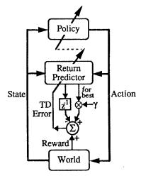
Figure 5. Q-learning Architecture. The line labeled "for best" is the prediction of return for the best action; the other output from the return predictor is the prediction of return for the action actually taken.
