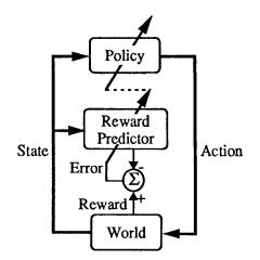
Figure 3. Reinforcement-Comparison Architecture.
